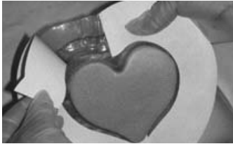
Fig. 2: Removing the release liner
